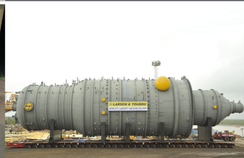
Heaviest Vacuum Column weighing 964 MT
