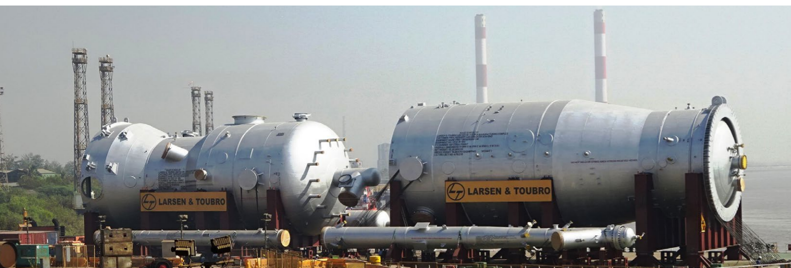
RAPID FCC Reactor-Regenerator Package, total 2 nos. weighing 8750 MT
