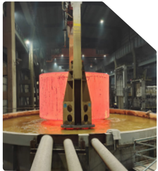
QUENCHING TANKS (Upto 0.8 Million litres)
