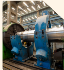
DEEP HOLE DRILLING Weight Upto 100 MT Max. Drilling Depth : 15000 mm
