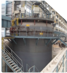
VACUUM INGOT CASTING (Upto 300 MT, H 2 <1 ppm)
