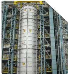
VERTICAL SHAFT FURNACE (Shafts Upto: Ø 2000mm, Height: 16m)
