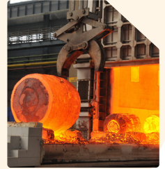
REHEATING & HEAT TREATMENT FURNACE (Upto 400 MT)
