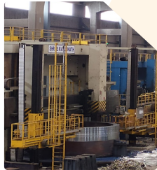
VERTICAL TURNING LATHE Weight Capacity (MT): Upto 250 MT Max Height (mm): Upto 5400
