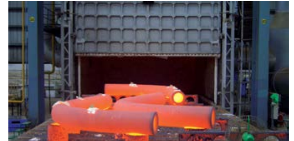
Heat Treatment Furnace
