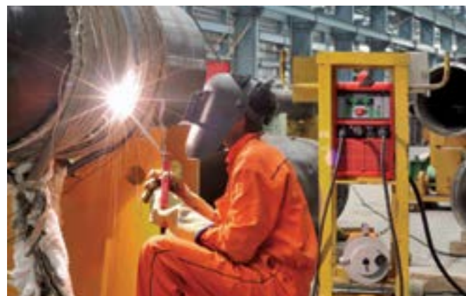
Shielded Metal /Gas Tungsten Arc Welding
