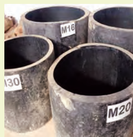
Scrap HDPE pipes are used for stacking nuts and bolts
